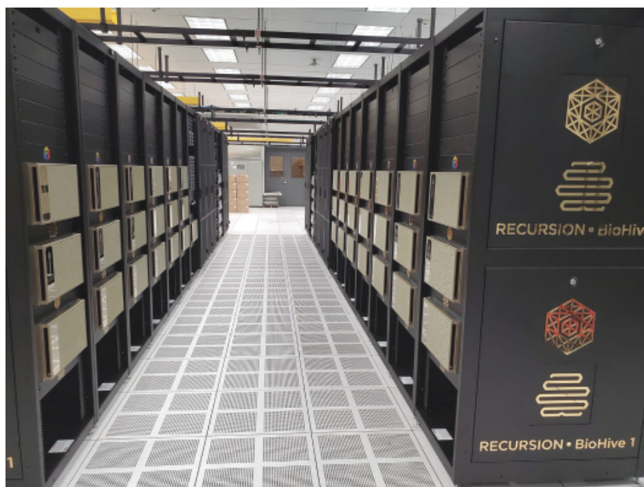
Figure 17. We believe BioHive-1 is one of the most powerful supercomputers dedicated wholly to drug discovery for a single company. BioHive-1 consists of 40 NVIDIA DGX A100 640GB nodes which further expands our capability to rapidly improve ML models.
