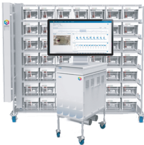
Figure 16. Our proprietary, scalable Smart Housing System for in vivo studies automatically collects and analyzes video and sensor data from all cages continuously.
