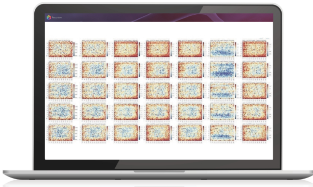
Figure 19. PlateWatch enables our team to identify potential irregularities and ensure high-quality data enters the Recursion Data Universe. PlateWatch automatically generates plate-level metrics and figures to assist our technicians in providing quality control for all phenomics experiments, rapidly identifying possible problematic plates and ensuring high-quality data enters the Recursion Data Universe. In this case, a set of plates that did not pass QC due to plate effects across various parameters were automatically flagged for further review.
