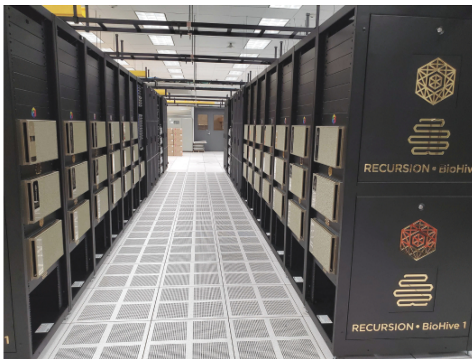
Figure 17. We believe BioHive-1 is one of the most powerful supercomputers dedicated wholly to drug discovery for a single company. BioHive-1 consists of 40 NVIDIA DGX A100 640GB nodes which further expands our capability to rapidly improve ML models.
