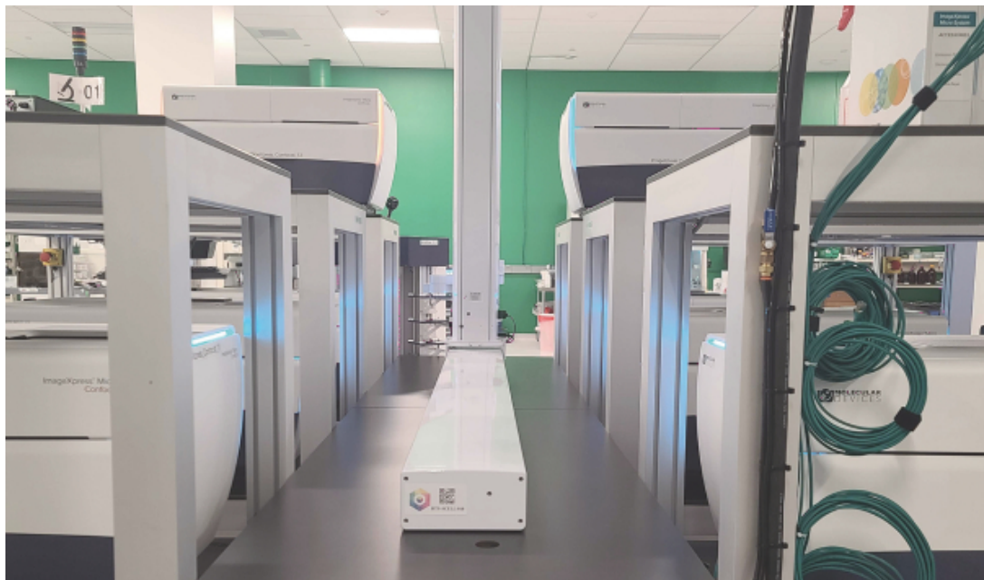
Figure 18. Our large installation of high-throughput microscopes. The 13 high-throughput automated microscopes are serviced by multiple robotic arms to enable near continuous imaging of our phenomic experiments. This imaging process not only increases the imaging speed but also reduces human intervention and error.
