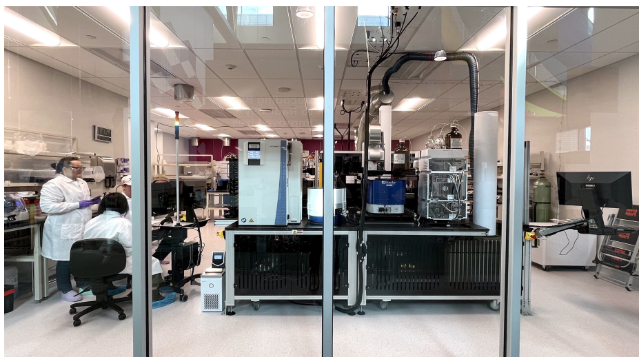
Figure 19. Recursion's automated DMPK module allows for automated assay execution across plasma protein binding, microsomal stability and cell permeability studies at scale and in both human and rodent cells to advance programs while generating state-of-the-art training data for ML and AI algorithm development. The system has been designed to potentially add new modules into the automated workflow, such as additional in vitro absorption, distribution, metabolism, excretion, and toxicity (ADMET) testing.
